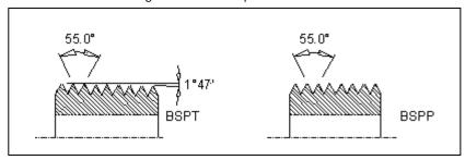
British Pipe threads have similar sizes as American Pipe threads BSP but they are not interchangeable due to different flank angle except at ½" and ¾" where both have same pitch.
