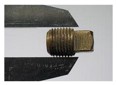
Note: The threaded pipe is tapered and so the Caliper touches the Pipe at two points
